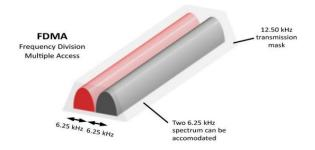
dPMR then goes one step further because it is a true narrowband technology that operates with less than half the bandwidth of normal PMR.
