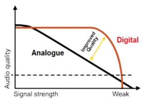
One area where digital can make a difference is at the edge of the radio coverage.
