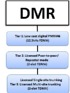
As the diagram shows, DMR is a full featured system capable of providing communications solutions ranging from license-free all the way up to multi-site trunking networks.
