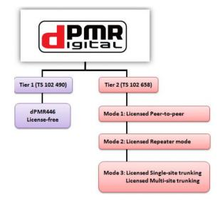
As the diagram shows, dPMR<sup>™</sup> is a full featured system capable of providing communications solutions ranging from license-free PMR446 all the way up to Mode 3 multi-site trunking networks.
